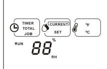
"CURRENT" HUMIDITY. When the machine is turned on, the default display function goes to "CURRENT" HUMIDITY. "CURRENT" wording in the square box will flash for 3 sec and 2 digits Relative Humidity figures display the current ambient humidity.
